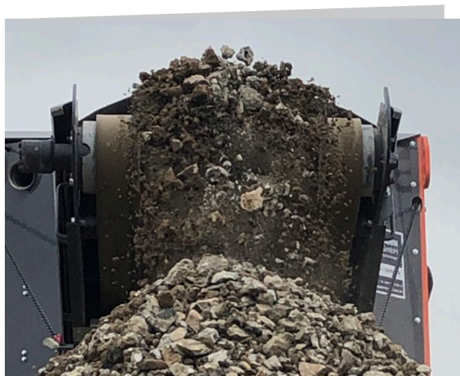
Stone crusher for processing waste directly on the construction
